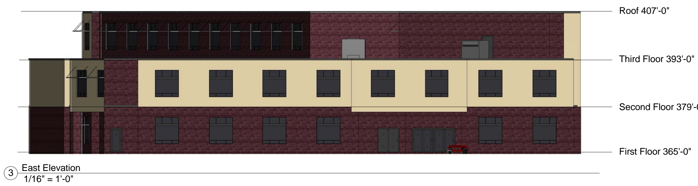
Figure 3 displays the East facade of the school building. The doors seen on the first floor are for emergency exit only. The door seen on the third floor leading to the roof is for access to perform maintenance on the mechanical equipment.
